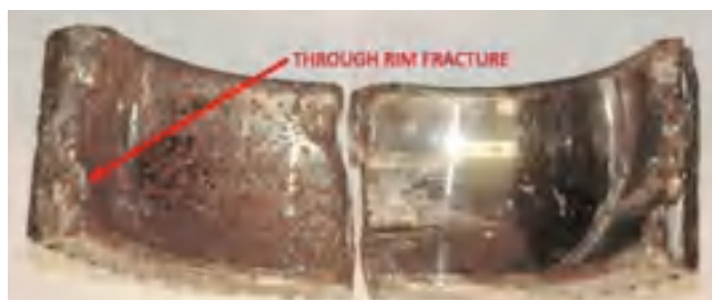
The two segments of the fractured second stage planet gear and an illustration of the second stage planet gear
