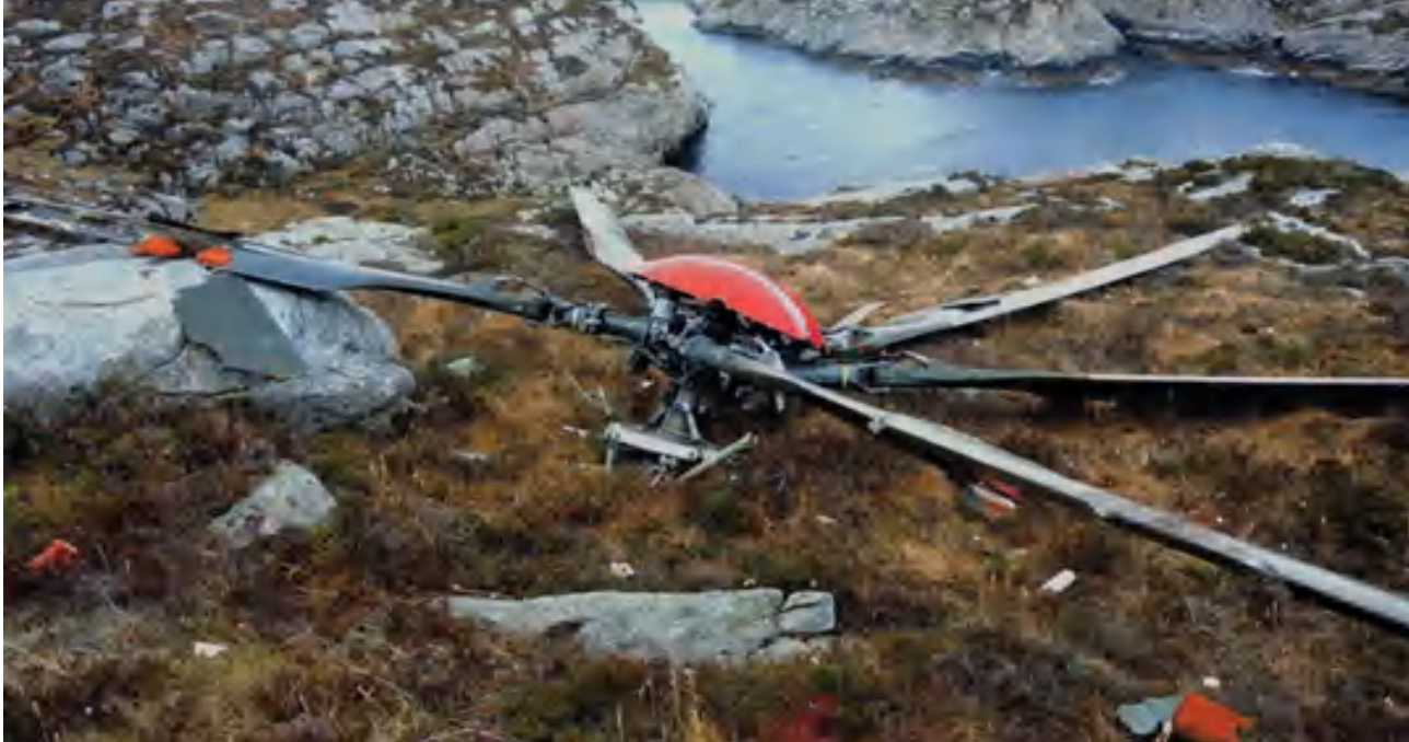
The main rotor and rear suspension bars as found on the island Storskora
