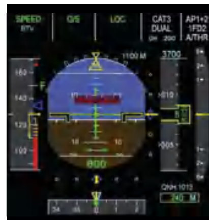
Windshear reactive warning displayed on PFD
