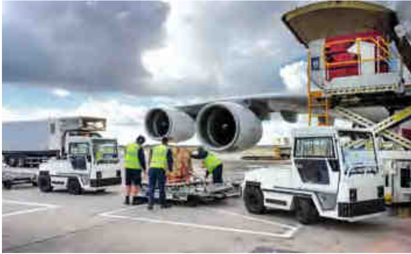
If the baggage handlers and ramp staff load the aircraft incorrectly then the out of trim condition could cause an incident or accident
