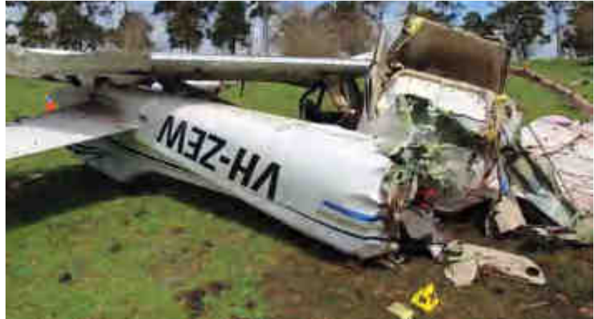
Figure 3: Accident site and wreckage of Cessna 172S Skyhawk SP, VH-ZEW
