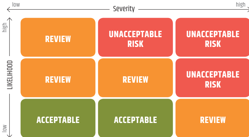
There are many ways an organization can assess risk. Here is one: a simple risk matrix. Each organization, however, should do what works for them.
