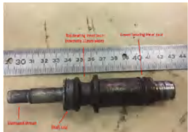
Oil cooling fan shaft during post-accident examination
