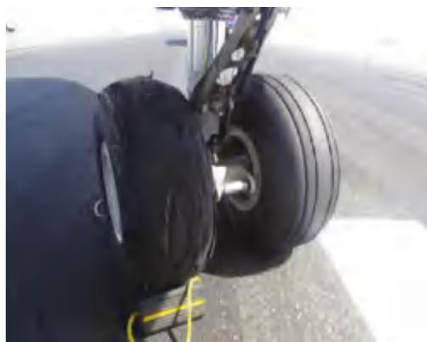
Figure 2. Nose gear No.1 tire damage
