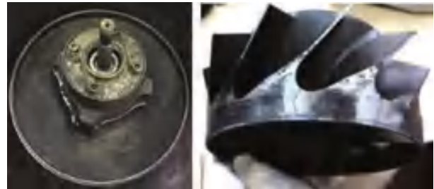
Fan shaft damage and damaged fan impeller
