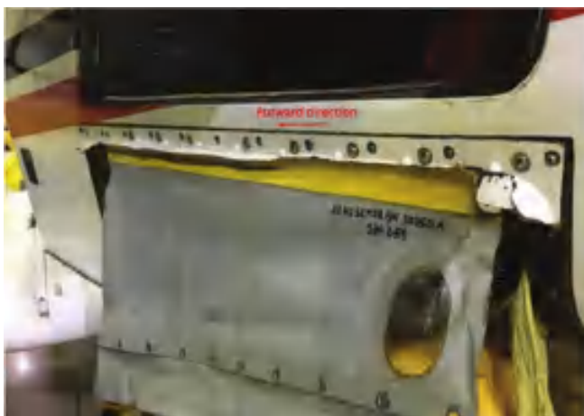
Left and right aft composite cover damage
