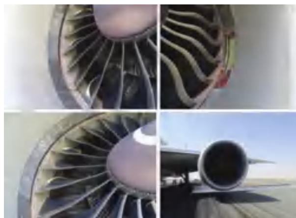
Figure 4. No.1 engine fan blade and Inlet damage
