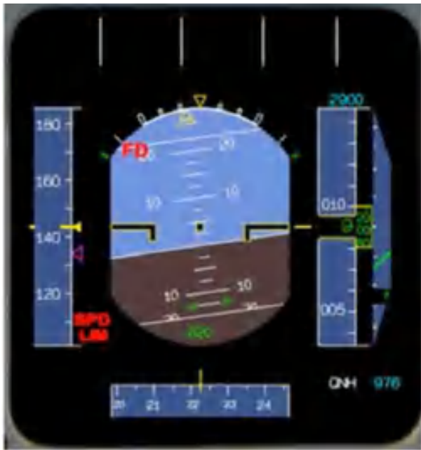
Figure 2. Primary Flight Display. [FD] and [SPD LIM] flags are displayed in red text. They respectively indicate the loss of Flight Director bars and the characteristic speed information.
