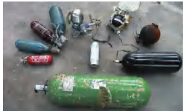
Figure 1: A selection of pressurized containers recovered from aircraft accidents
