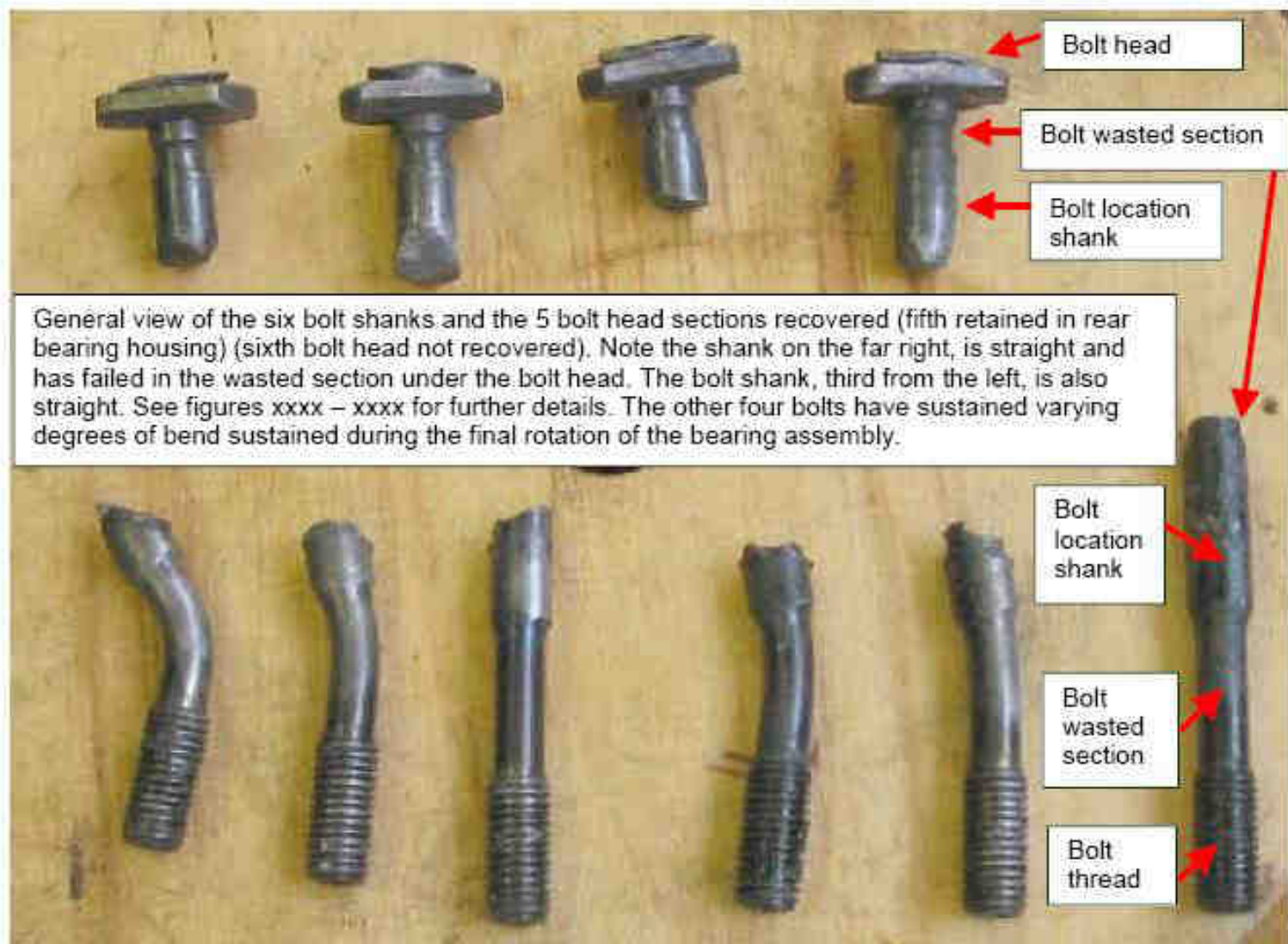
Figure 43. Showing the general condition of the bolts. One bolt head was still located in the rear bearing housing and the bolt head of the straight bolt has not been located.
