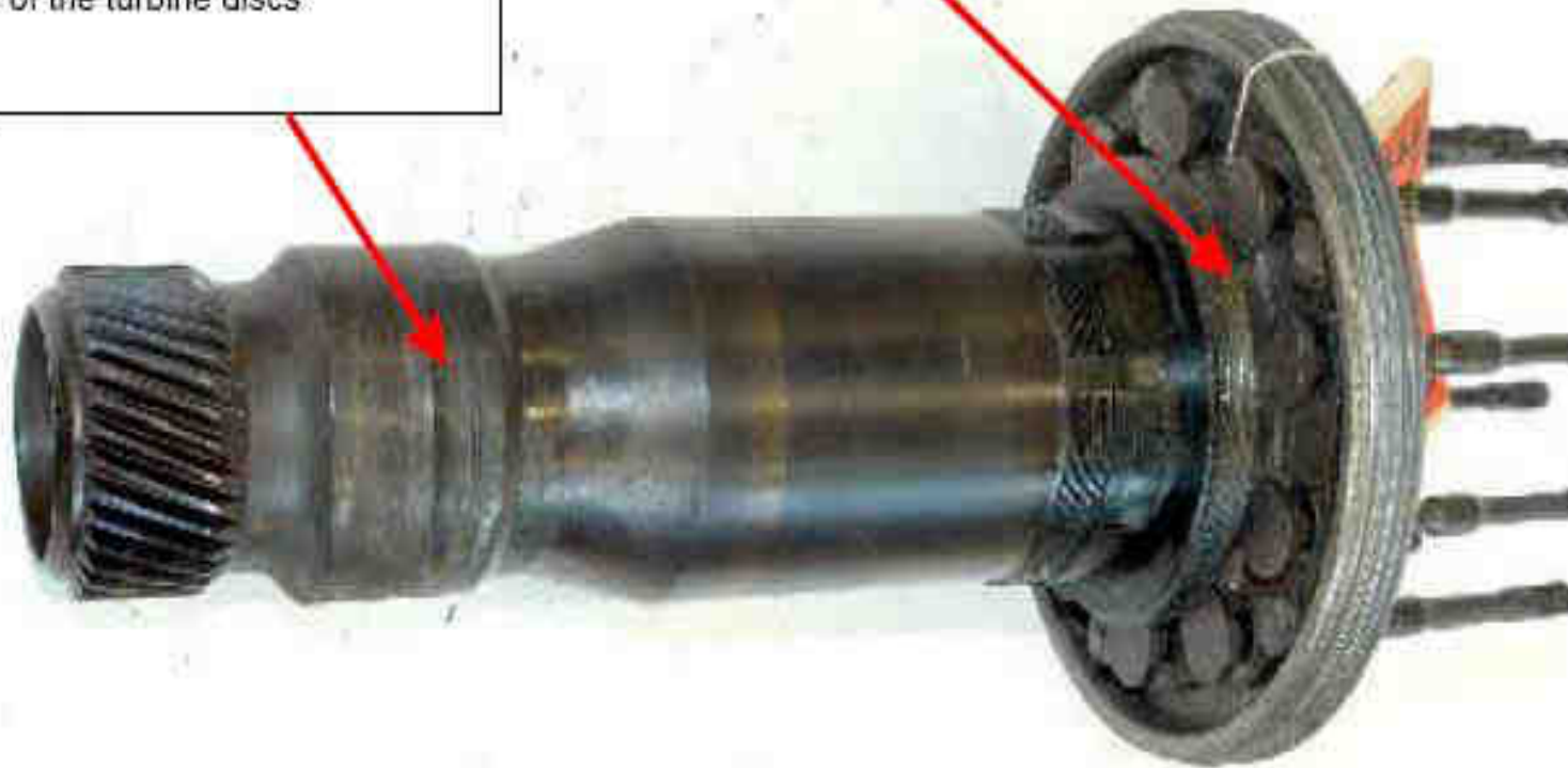
Figure 20. LPT shaft. View showing position and arc of heavy rub to the plain bearing journal.
